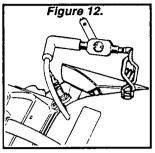
NOTE: The Ignition Sensor is mounted to the generator's Stator Adapter. To replace the Sensor, disassembly of the generator and removal of the Stator will be necessary.
